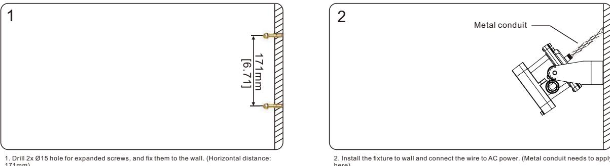
1. Drill 2x Ø15 hole for expanded screws, and fix them to the wall. (Horizontal distance: 171mm)
