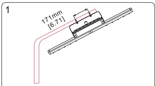
1. Drill 2x Ø15 holes for fixing screws.
