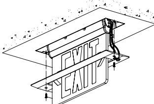
The recess kit allows for the standard surface mount SEEXLRN to be easily recessed into a ceiling or a wall. The standard unit snaps into the recessed backbox and is securely held in place while wiring is completed.
